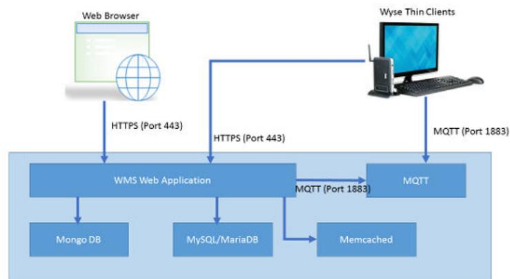
Figure 1. Architecture de la solution Wyse Management Suite
